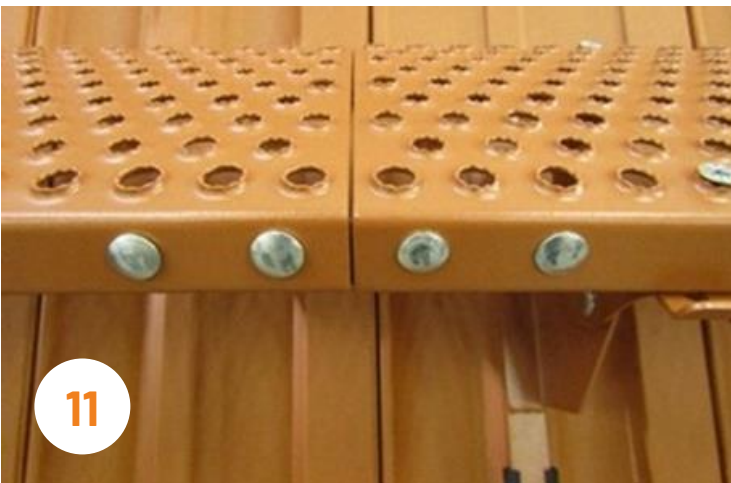
Place the metal plates to the inner side of the grid (both side) and fix it with 4-4 pcs of screws! Use a size 13 wrench!
